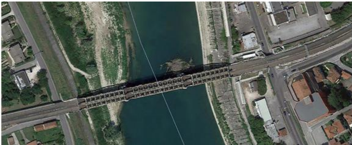
Figure 1. Satellite image of a large wood accumulation at a railway bridge crossing the River Tagliamento in Latisana (Italy). Source: Google Earth. Image: Landsat/Copernicus (from Panici et al., 2020 )
